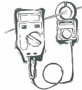
Combination with clamp on probe allows current measurement
